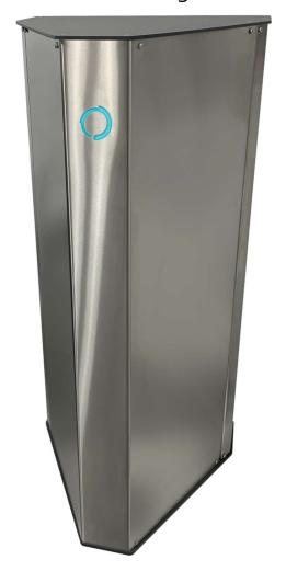
The Torrent 9000 is a compact RO-based (reverse osmosis) water purification system that has been designed to provide 95%+ TDS reduction for demanding applications. It accomplishes this while producing a very small amount of waste water, unlike traditional RO systems. The Torrent 9000 is also a water softener, reducing hardness by up to 98% without the use of salt.
